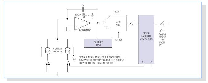
Figure 2. This circuit configuration is an analog integrating servo loop.
