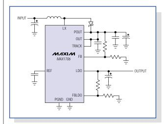
Figure 6. As a third option for maintaining regulation when the input range overlaps the output voltage, this IC combines a switching regulator (for step up) and a linear regulator (for step down).
