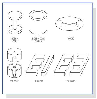
Figure 10. Different core geometries offer trade-offs among energy storage, field emission, and ease of assembly. All can be gapped.
