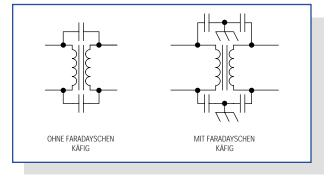
Figure 8. A Faraday shield between primary and secondary blocks common-mode noise that would otherwise pass through the transformer's parasitic interwinding capacitance.
