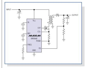
Figure 4. A flyback regulator maintains regulation for inputs that range above and below the output voltage.
