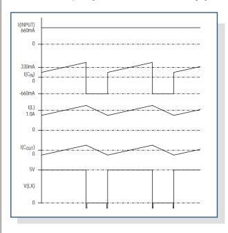
Figure 2. These waveforms from the Figure 1 circuit are based on an assumption of ideal components.
