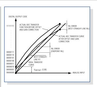
Figure 1b. Best-straight-line and endpoint fit are two possible ways to define the linearity characteristic of an ADC.
