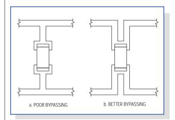
Figure 12. Poor bypass connections (a) add trace inductance and resistance to the capacitor. In the better connection (b), trace parasitics add to the capacitor's filter action.
