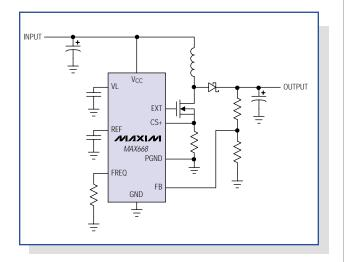
Figure 3. This step-up switching regulator lacks synchronous rectification, but is otherwise similar to the step-down type, with inputs and outputs swapped.
