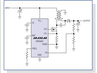
Figure 5. Otherwise similar to a flyback regulator, the SEPIC has continuous primary and secondary currents that generate less noise.
