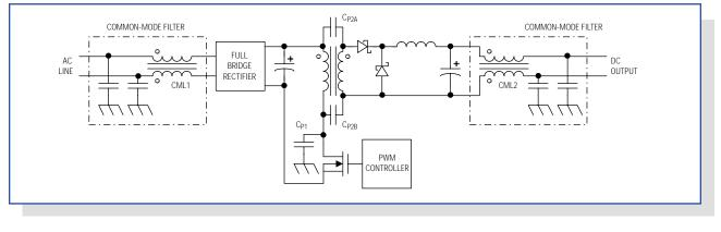
Figure 7. Common-mode filters in this typical off-line power supply reduce noise common to both sides of the input and output.
