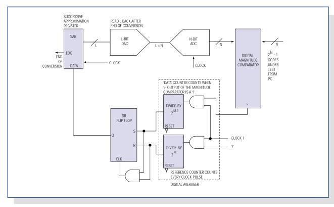
Figure 5. Successive approximation and a DAC configuration replace the integrator section of the analog servo loop.
