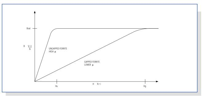
Figure 9. Gapping a ferrite core forces magnetic flux out of the core and allows the inductor or transformer to store energy in a field surrounding the device.
