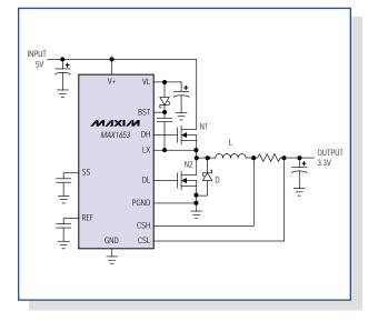
Figure 1. This illustrative step-down switching regulator features an external switching transistor (N1) and synchronous rectifier (N2).
