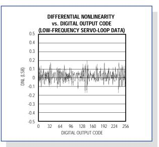
Figure 4b. This plot shows typical DNL for the MAX108, captured with the analog integrating servo loop.
