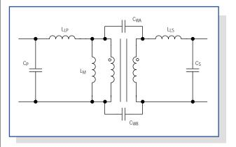
Figure 11. Parasitic elements in the equivalent model for a transformer modify its ideal behavior.
