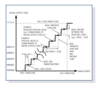
Figure 1a. To guarantee no missing codes and a monotonic transfer function, an ADC's DNL must be  $\leq$  1LSB.
